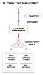
Figure 25: 6 Phase / 12 **Pulse System**
