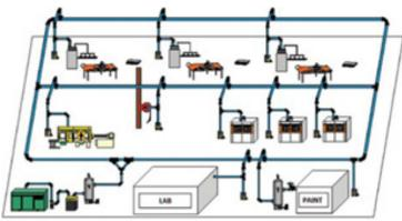
Figure 14: Pictorial representation of ring main system
