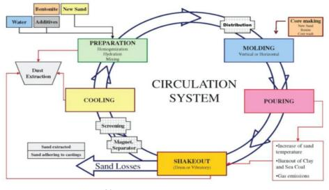
Figure 21: Typical sand handling system in foundries
