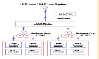
Figure 26: 12 Phase / 24 Pulse system
